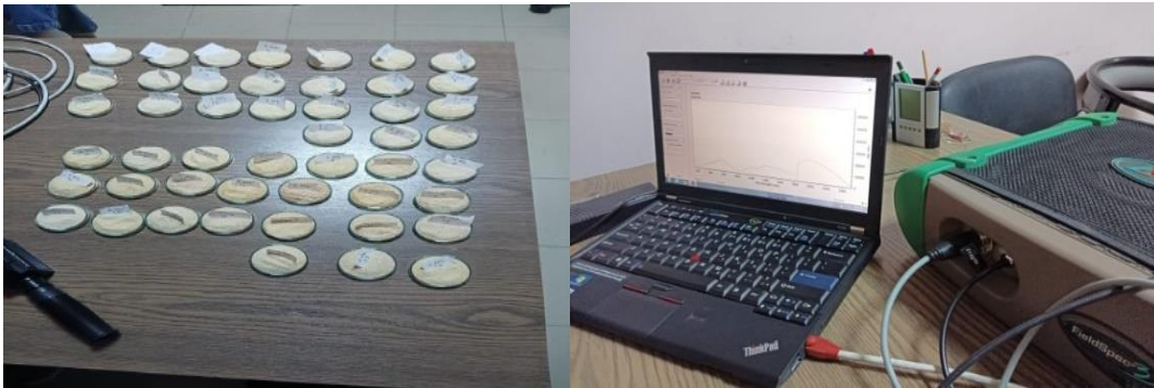
Figure 3. Taking reflections of soil samples with the Field Spec III Spectroradiometer instrument
